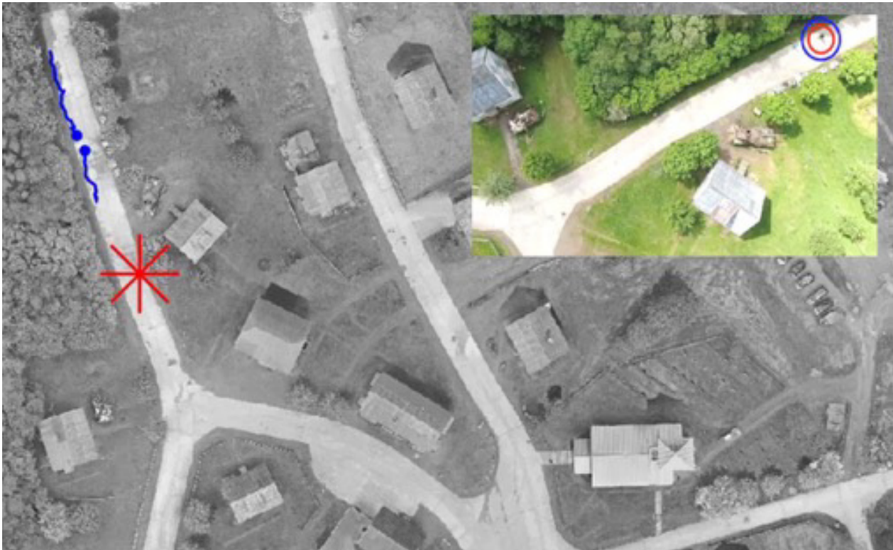
Figure 8: Orthographic photograph of Demonstration Area. The UAV is marked with a red star and the motion of two persons on the ground are marked with blue lines. An image from the UAV is shown in color, with a detected person marked with concentric rings.
