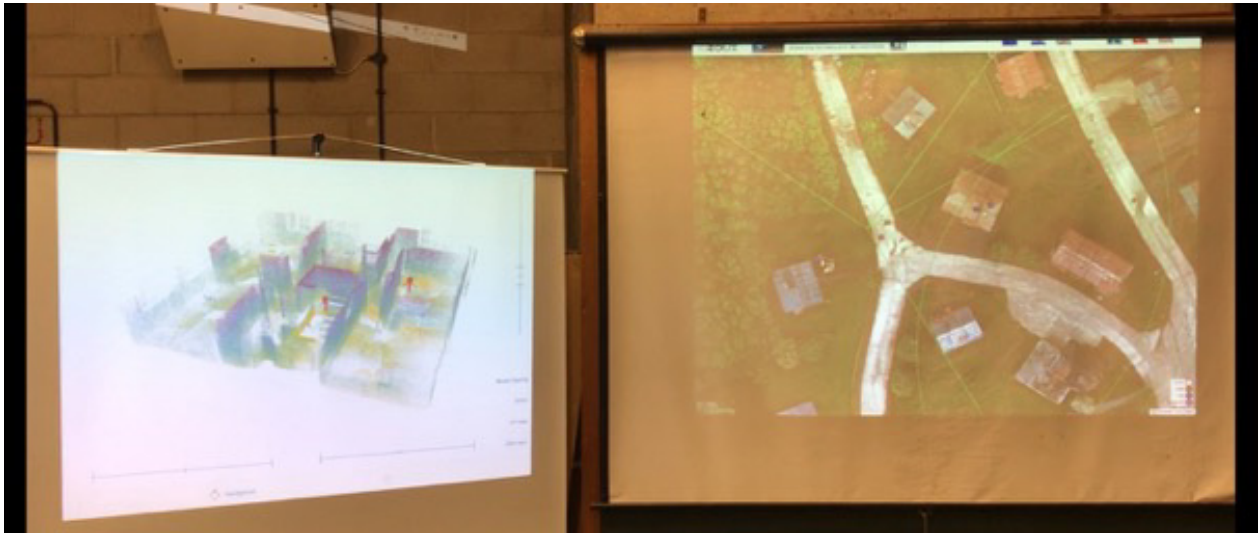
Figure 5: Actual picture of the Mission C2 Center visualization system highlighting the real-time simultaneous indoor/outdoor tracking in both a 2D top view on the map for general SA (right screen) and in 3D for better micro location awareness for indoor tracking.
