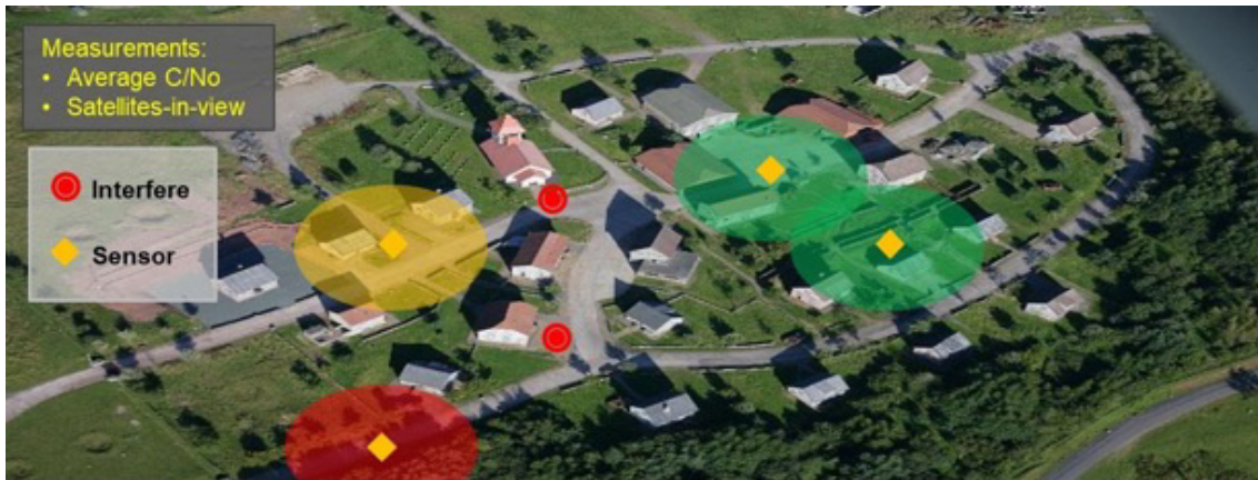
Figure 29: GNSS monitoring system C2 display.
