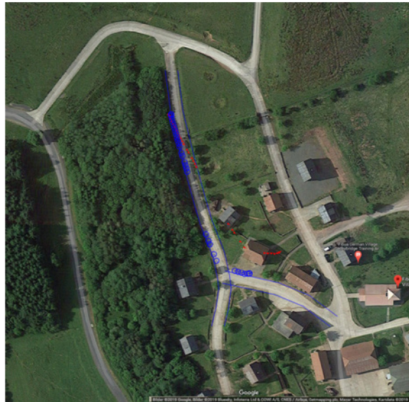
Figure 11: Navigation supported by track-sharing from UAV. Data collected during the pre-trials, where red dots represent dead-reckoning by a foot-mounted system without support. The blue circles is the result after fusion with tracking data from the UAV (orthophoto background © Google & Bluesky).
