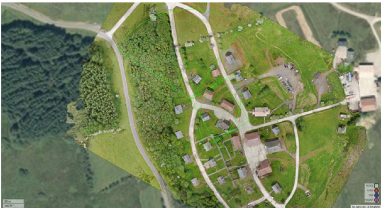
Figure 3: Map screen of the demo range in the Mission C2 Center software with satellite image in the back and high resolution (up to date) map created with drone overfly in the front.
